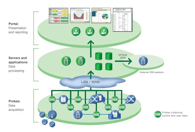
The MasterClaw system is based on a three-layer architecture with distributed intelligence: The data acquisition layer with distributed probes for end-to-end coverage, the data processing layer with servers and applications, and the presentation layer with an advanced, web-based GUI portal.
